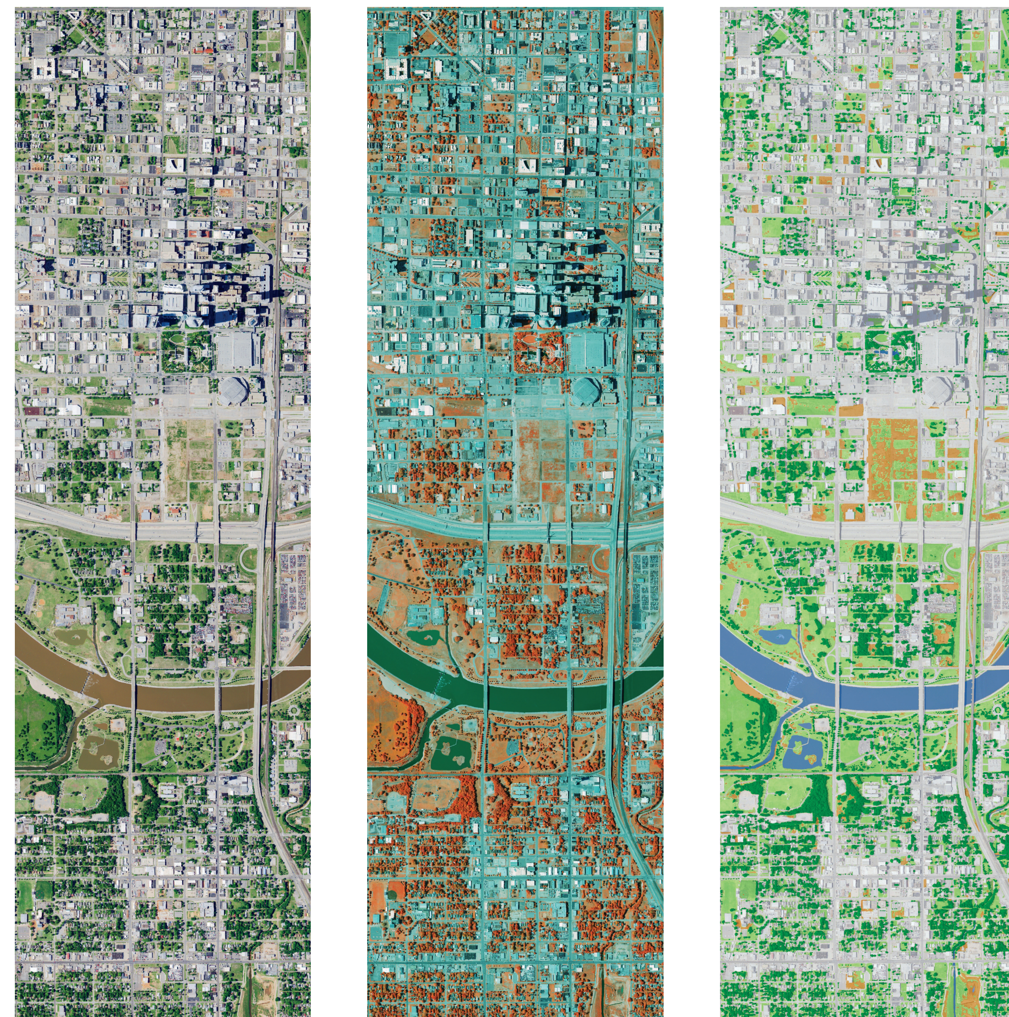
High-resolution aerial imagery (left) was used to remotely identify existing land cover. Infrared technology delineated living vegetation including tree canopy (middle). Remote sensing software identified and mapped tree canopy and other land cover (right).
