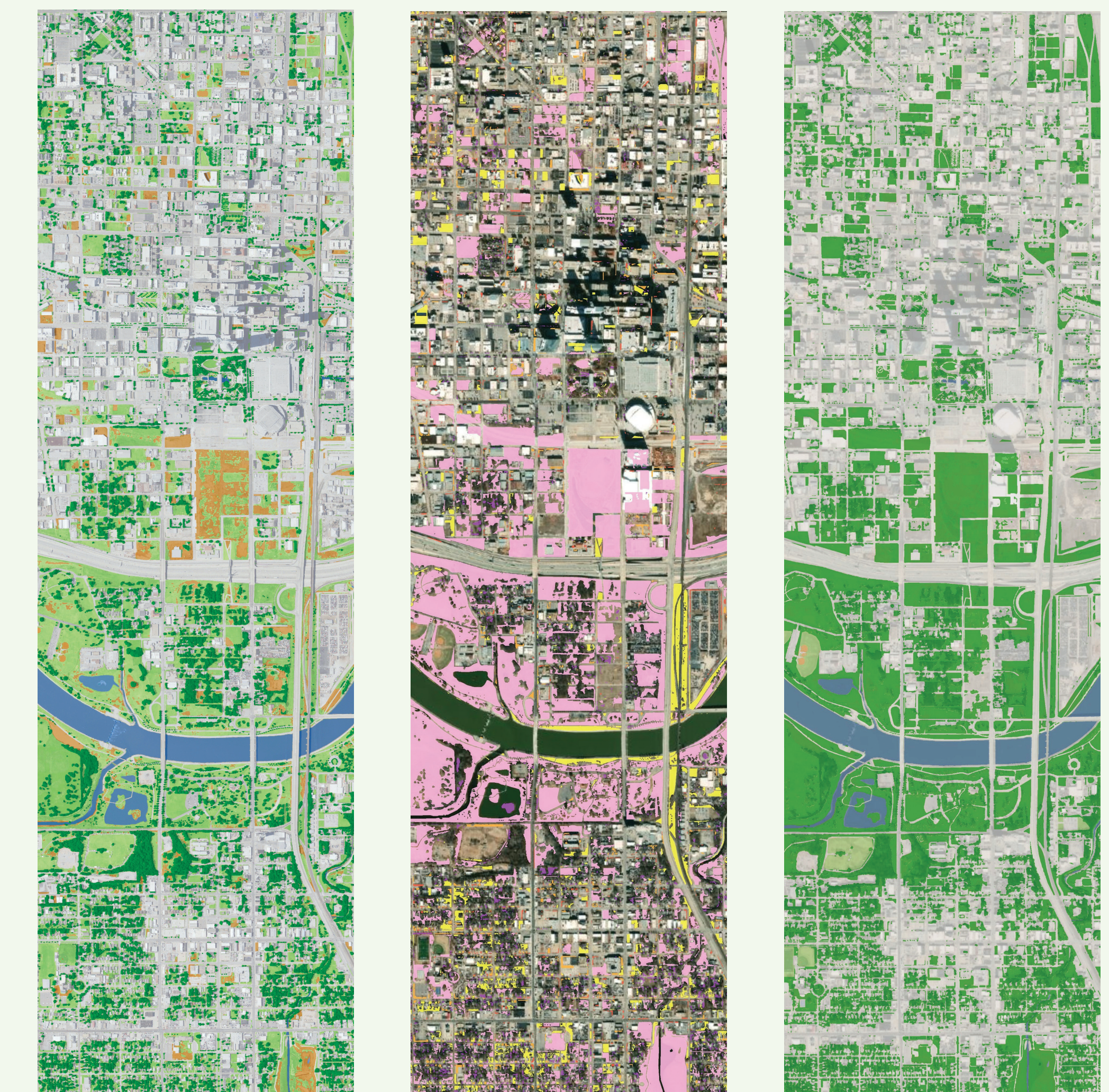
Existing land cover in Oklahoma City (left), areas of planting potential for Urban Heat Island impact (middle), and the region if all priority areas were planted on (right). Planting in areas with high percentages of impervious surfaces may alleviate the urban heat island effect.
